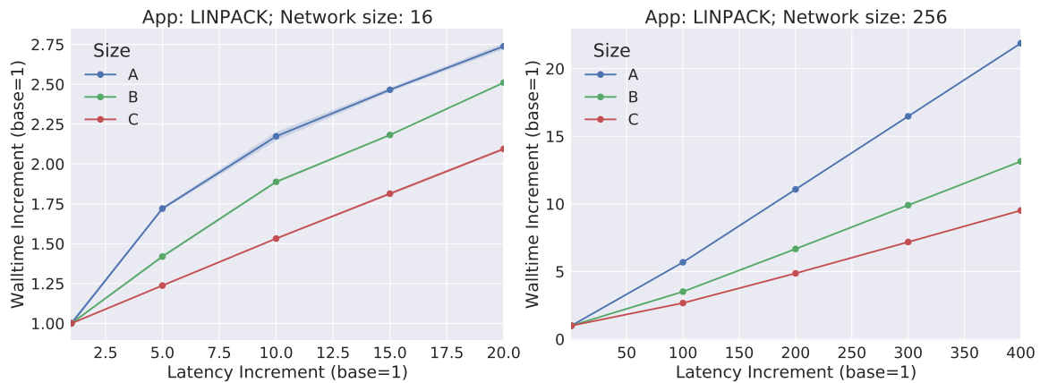
Figure 3.10: Slowdown on the isles topologies as a function of the increment in the latency of the distinguished link in LINPACK.
