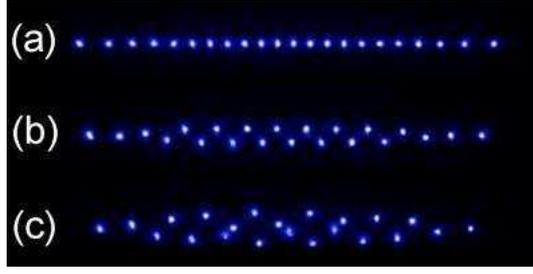
Figure 3.2: Different equilibrium structures: (a) linear string of ions, (b) two-dimensional zig-zag structure and (c) three-dimensional helix. Images like these are obtained by irradiating the ions with laser light of the appropriate frequency and detecting its fluorescence with a CCD camera.
