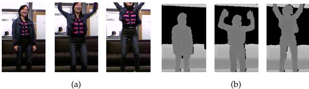
Figure 1.2: RGB (1.2a) and depth (1.2b) sequences for an instance of the cheer up action.
