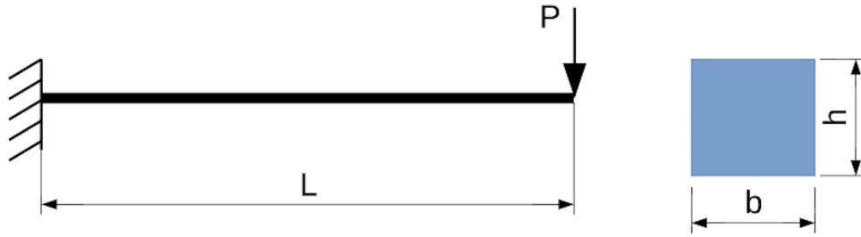
Fig. 6.3: Schematic representation of a bending test with a punctual load.
