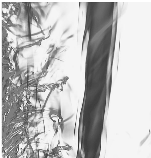
Figure 3. Zoom on vorticity intensity, when strong, at late times in the same simulation as in figure 2. The colocation of laminar structures, BCV and of a tangle of vortex filaments with more complex paths and at smaller scale, to the left of the BCV, is clear. The BCV columns, different from Taylor columns (see text) are updraft cyclonic vortices that are fully helical (figure 2) and thus live for a long time, whereas the small-scale vortices are more evanescent, living for a couple of eddy turnover times. Note two less-intense and inter-twined smaller multiple vertical vortex cores to the left.
