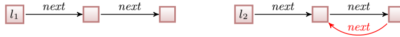
Fig. 5: Structures l_1 and l_2 are built with linked list nodes; l_2 is not acyclic .
