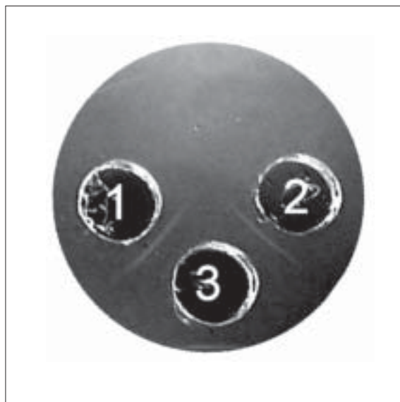
Fig. 4.– Ouchterlony double diffusion test. Immunodiffusion of PLA 2 (1mg.ml -1 ) (3) against anti-sera raised in rabbits (2) and IgG anti-PLA 2 (1).
