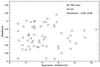
**Fig. 3.** Abundance vs. Equivalent width for 60 FeII lines, using the gf values from Martin et al. (MF) plus Kurucz values (KX). The minimum slope is obtained for a value of 2.0 kG.
